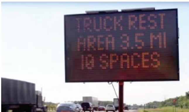
When a truck approaches a facility, the system provides a final notification regarding availability so that the driver can avoid entering and searching the facility if all spaces have been filled. When a truck enters a space, the system reduces the available count by one. When a truck exits a space, the system increases the space-available count by one. In each case, the
